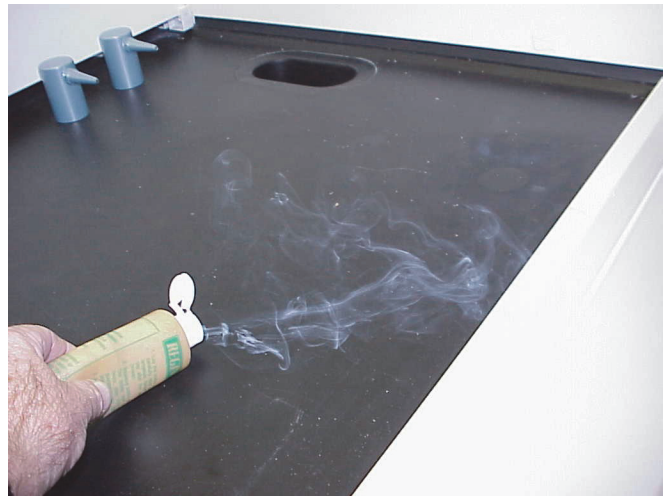
FIGURE 3.3 Reverse airflow as demonstrated by smoke visualization.
