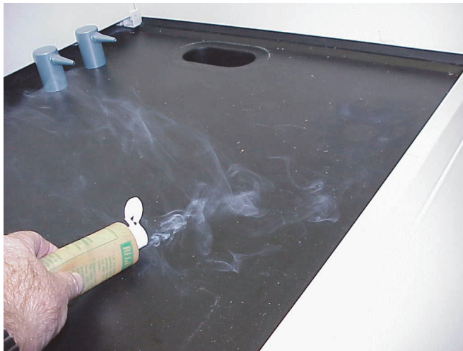
FIGURE 3.2 Lazy airflow as demonstrated by smoke visualization.
